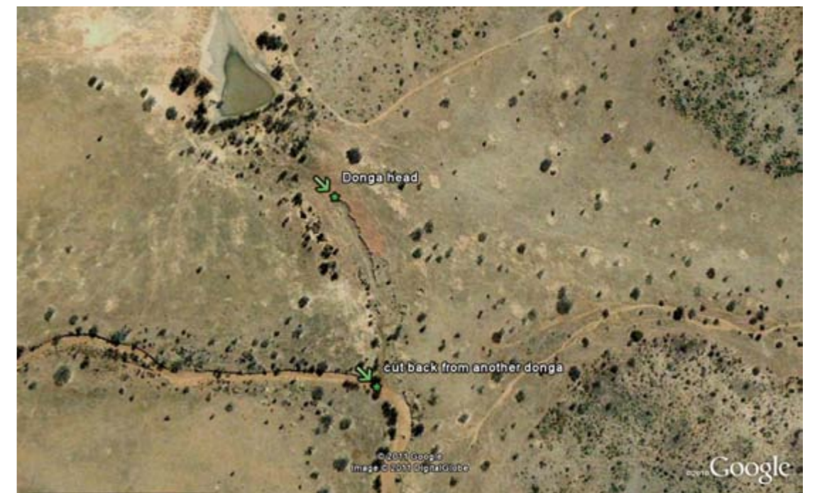
Figure 3. The donga head cutting back towards the Vlagte Dam on Farm Krumhuk has cut back from a more deeply cut down channel that turns sharply west. This deeper channel also ends upslope in gully heads indicating that it is not a natural drainage feature either. The concentrated overflow from Vlagte Dam has spilled over into the incised channel and set off the current donga head cutting back to the dam's spillway. The old, unchanneled water course is parallel to the donga, as indicated by the line of trees.
